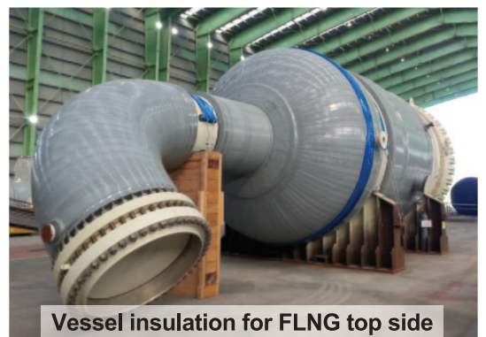
Pipe insulation for FLNG top side
