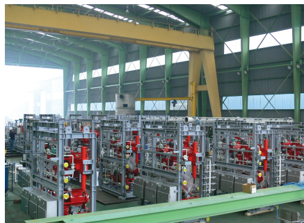
Valve skid for FLNG
