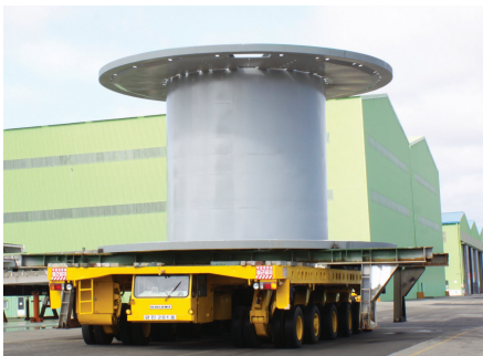
Reel for pipe laying vessel
